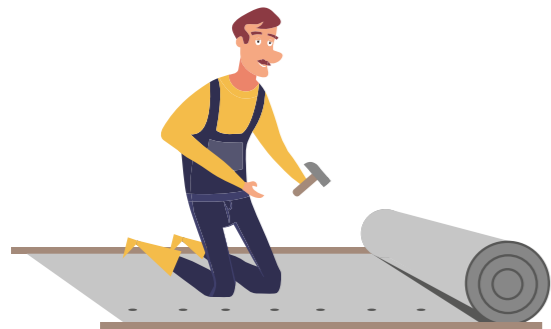
Nail or peg the weed membrane to the sand sub base
