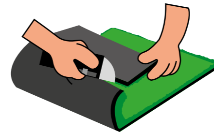
Cut carefully into the backing and trim the artificial grass
